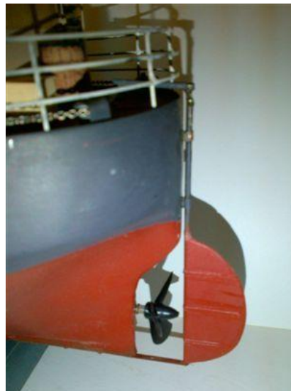
Figure E The completed rudder on Steve's Clyde Puffer .
