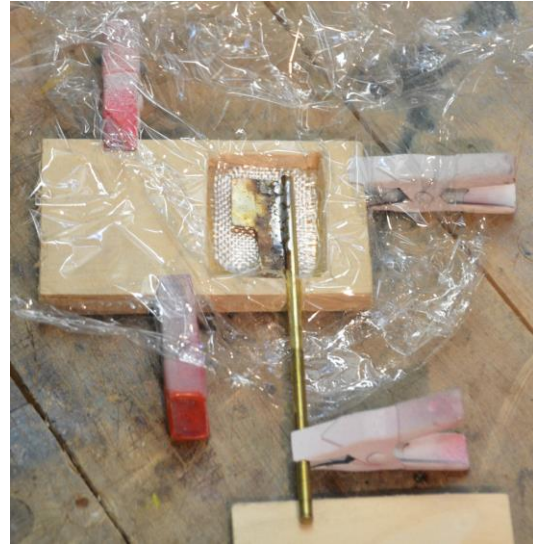
Figure K. The mould ready for the epoxy. In this photo a second piece of wood is used for the base of the mould and the two clamped together.
