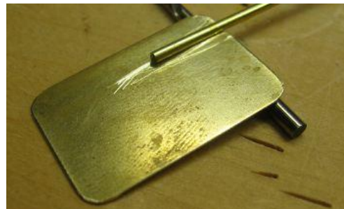
Figure C. The rod set in the groove in the blade ready for soldering.
