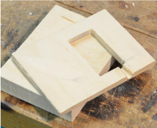
Figure J. A mould prepared from a piece of wood.
